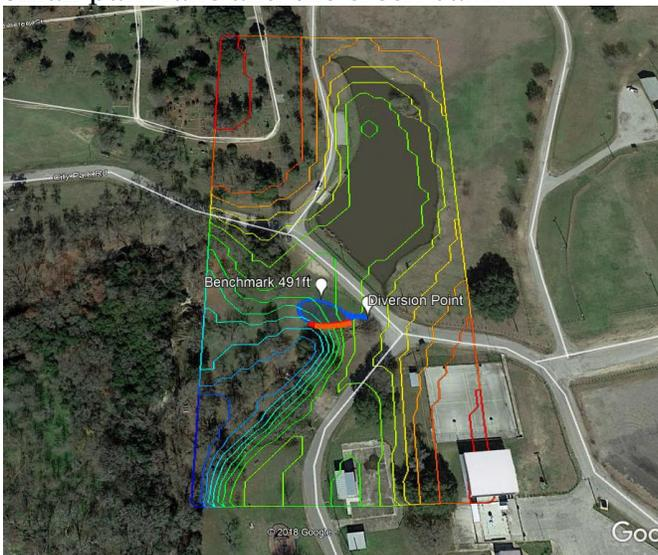
*Fig 1. Google Earth™ image of the City Park Rain Garden site with topographic contours overlain and diversion point and garden site identified.*
